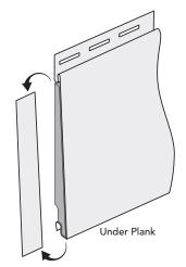
• Overlap Over Plank on top of Under Plank.
