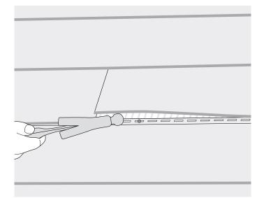
8 Remove shims and starting at overlap, apply upward pressure to the bottom lock leg to engage stack lock into top lock of replacement plank.
