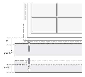
• When measuring the plank horizontal cut above obstacles, hook tape measure onto the backside of the receiving channel and measure to the top of the plank face of previously installed plank (past nail hem). Transfer measurement plus 3/4" to the cladding plank by pulling tape measure from the bottom of plank and mark measurement plus 3/4". Remove bottom of plank to the width of obstacle plus clearance (1/4" or 3/8") on both sides of obstacle.
