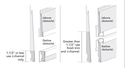
– When measuring the plank horizontal cut under obstacles, place tape measure into the backside of the receiving channel and measure to the top of the plank face of previously installed plank (past nail hem). Transfer measurement plus 1/4" to the cladding plank by pulling tape measure from the bottom of plank and mark measurement plus 1/4". Remove top of plank to the width of obstacle plus clearance (1/4" or 3/8") on both sides of obstacle.
