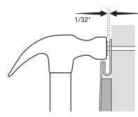
Allow 1/32" clearance between fastener head and nailing hem for expansion.
