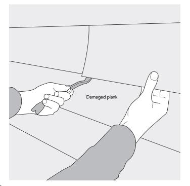
4 Place wood shims behind the cladding planks allowing more room to the nail hem of damaged plank.
