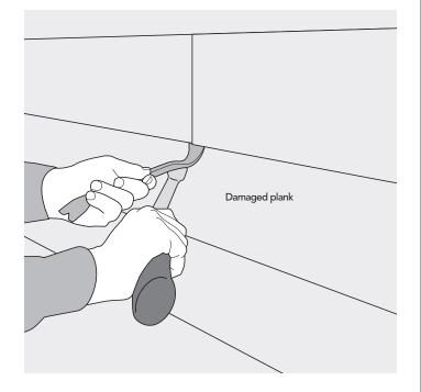
3 Using a hammer, tap up on pry bar to unlock stack lock from the top lock of damaged plank. Repeat this step, working away from the overlap until stack lock is unlocked across the length of damaged plank.
