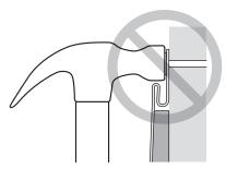
Do not drive the head of fastener tightly against the cladding nail hem.
